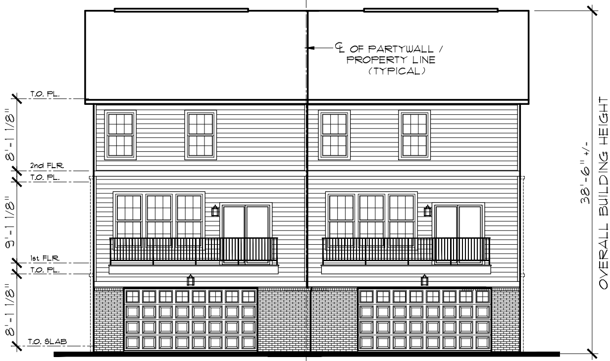
REAR ELEVATION 2-UNIT REAR-LOAD BUILDING
