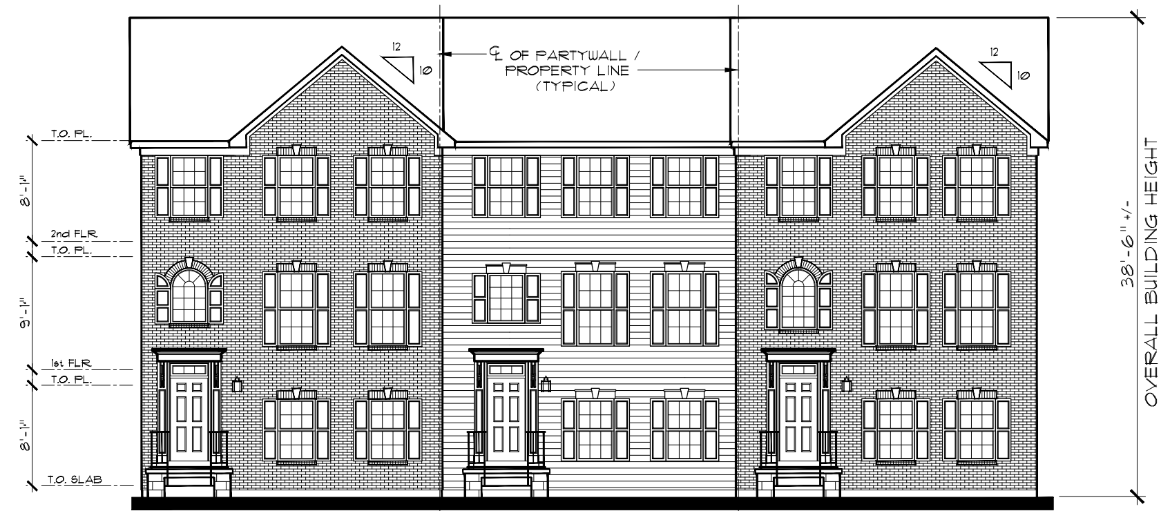
FRONT ELEVATION 3-UNIT REAR-LOAD BUILDING
