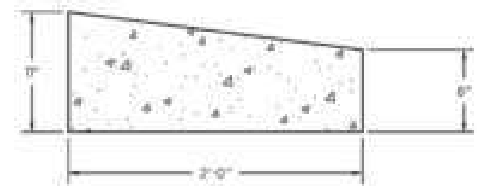
CONCRETE SLOPED CURB - FOR ROUNDABOUTS Not to Scale
