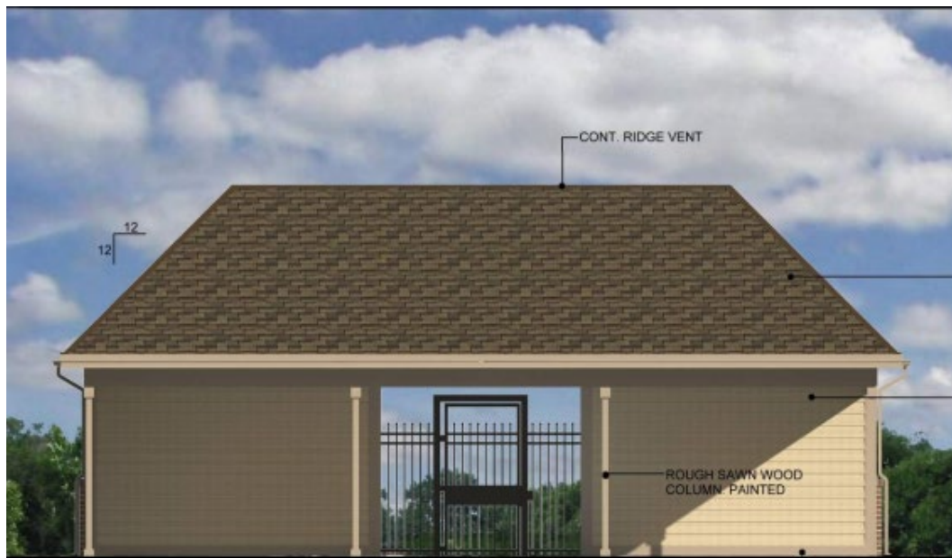
Rear elevation of the pool house.
