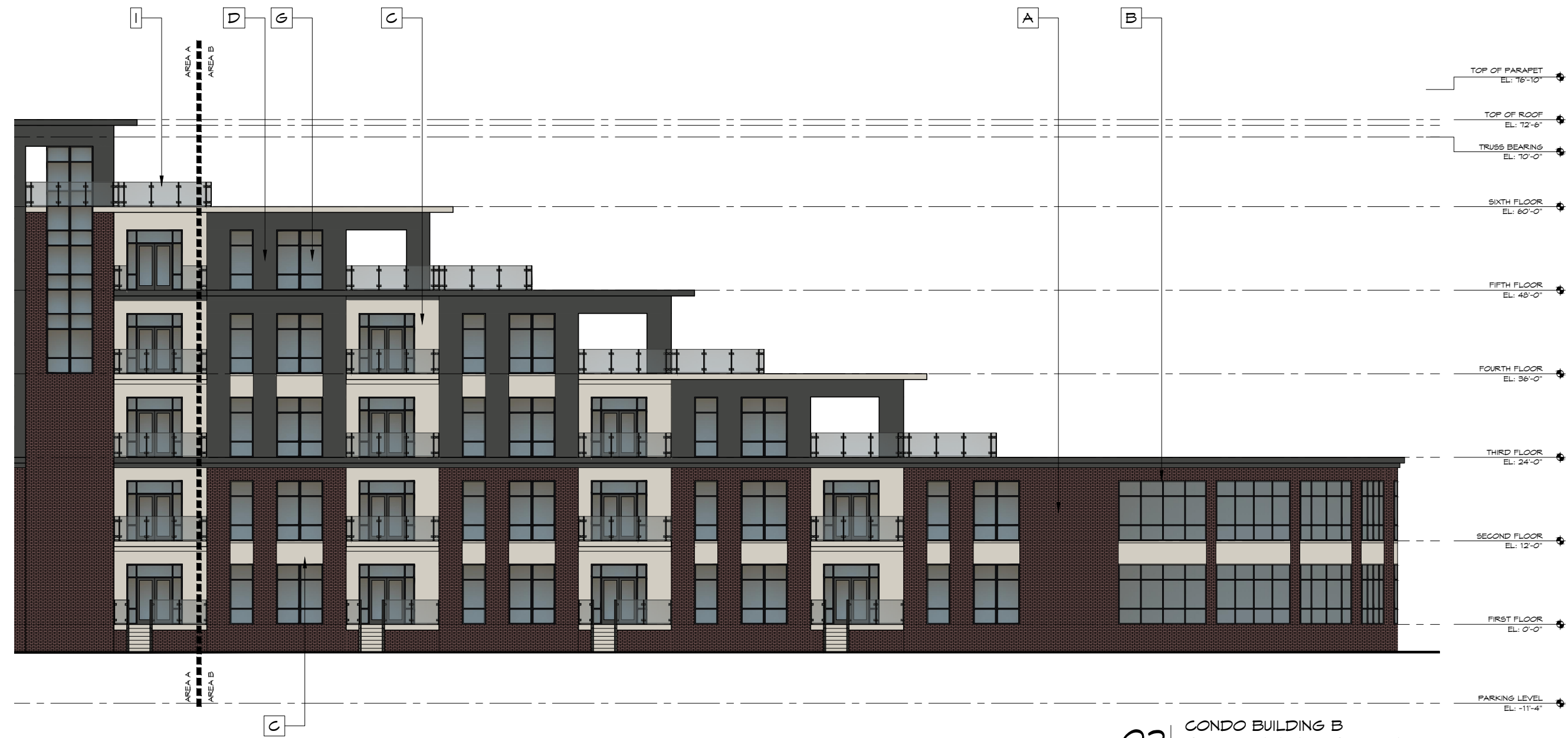
02 CONDO BUILDING B TRAIL SIDE ELEVATION AREA B SCALE: 1/8" = 1'-0"
