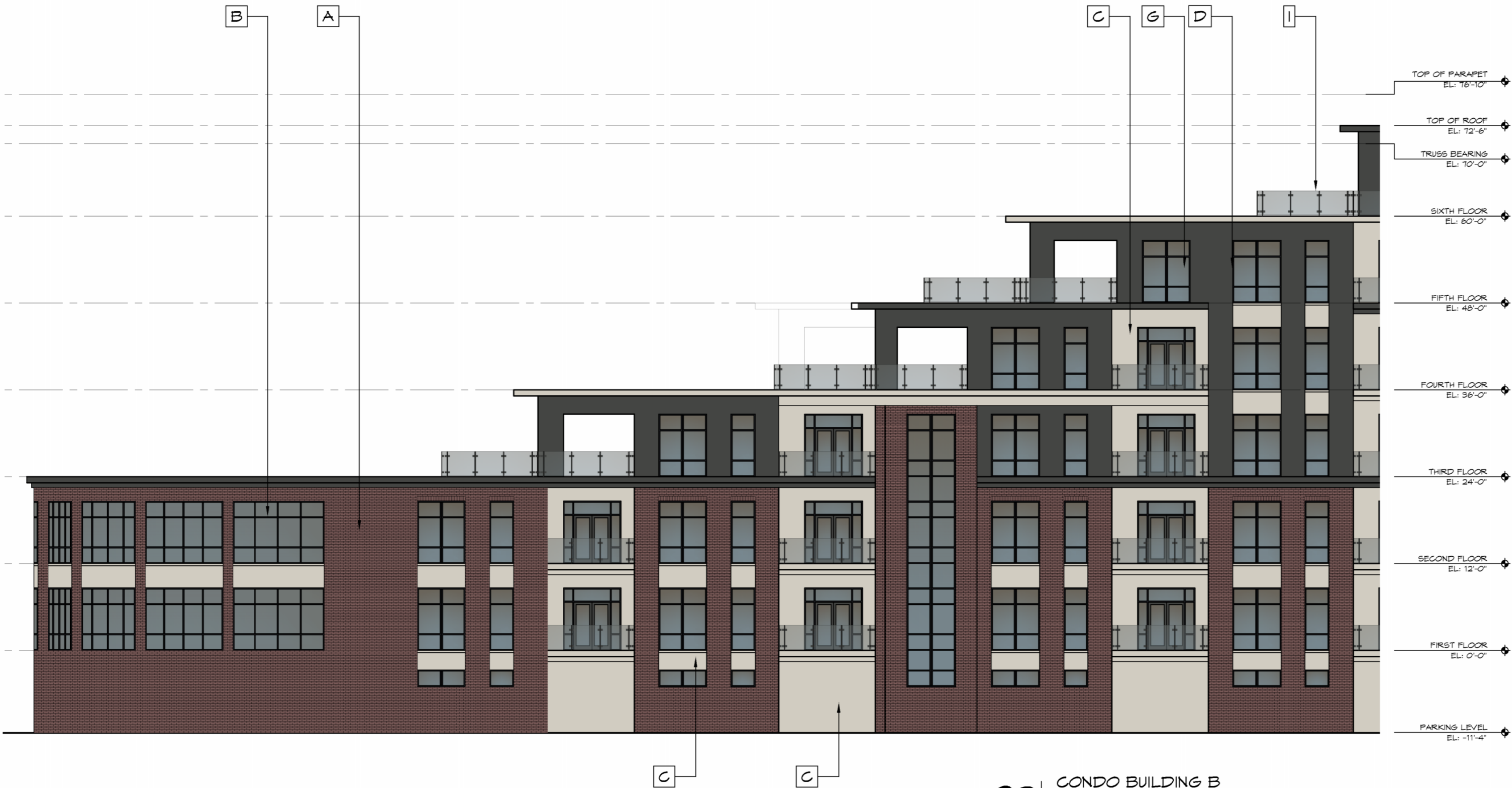
02 CONDO BUILDING B COURTYARD SIDE ELEVATION AREA B SCALE: 1/8" = 1'-0"
