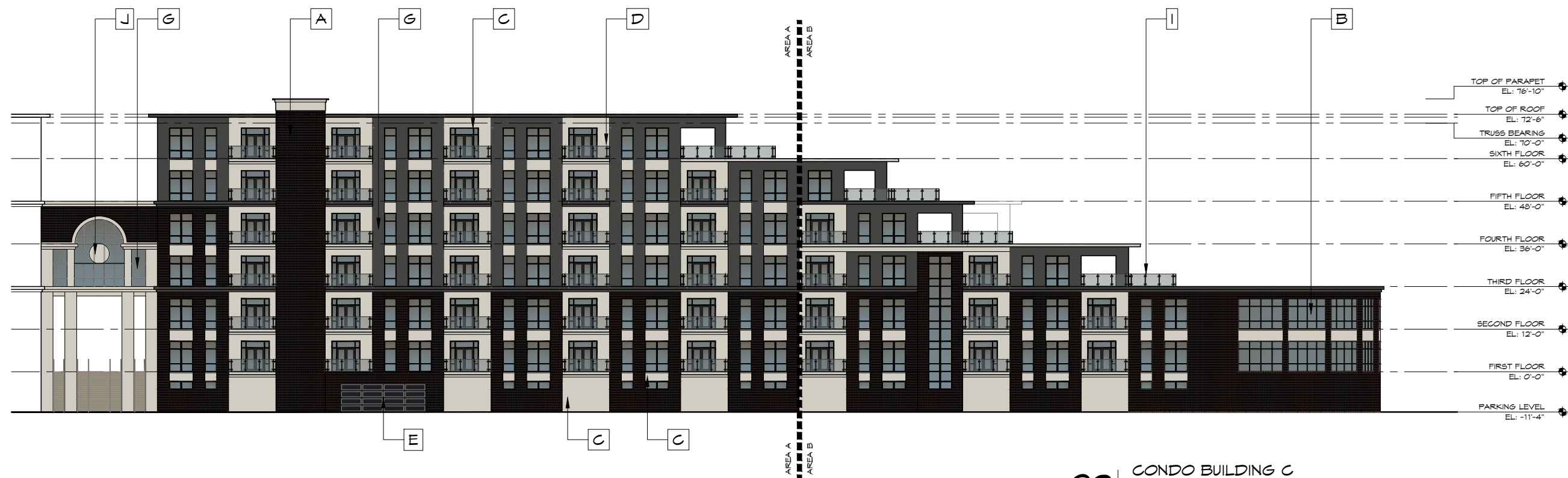
02 CONDO BUILDING C OVERALL COURTYARD SIDE ELEVATION SCALE: 1/16" = 1'-0"
