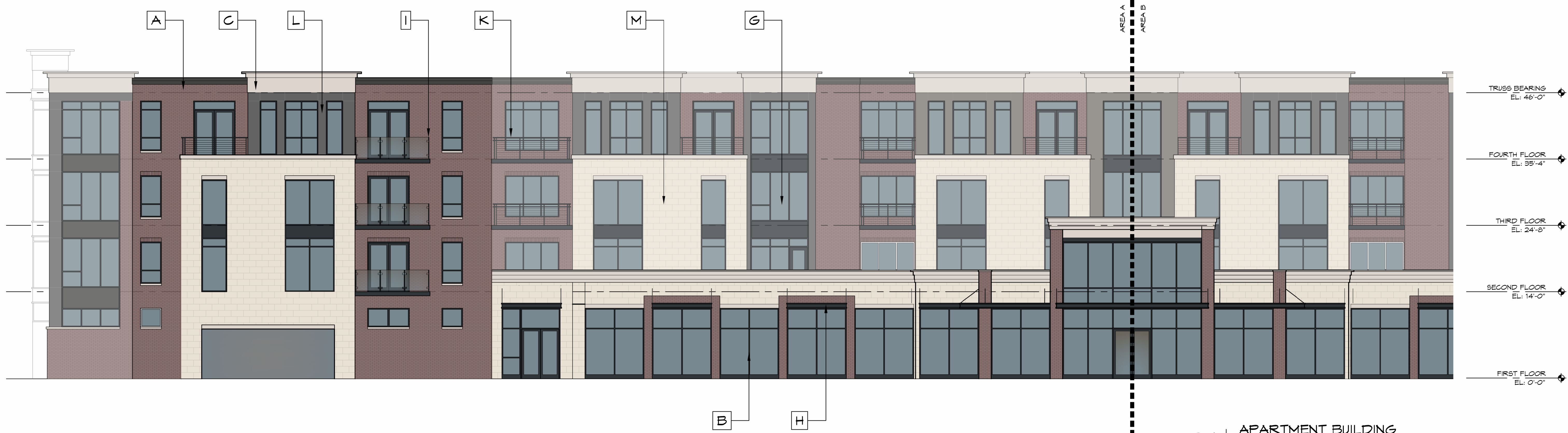
01 APARTMENT BUILDING SOUTH ELEVATION AREA A SCALE: 1/8" = 1'-0"
