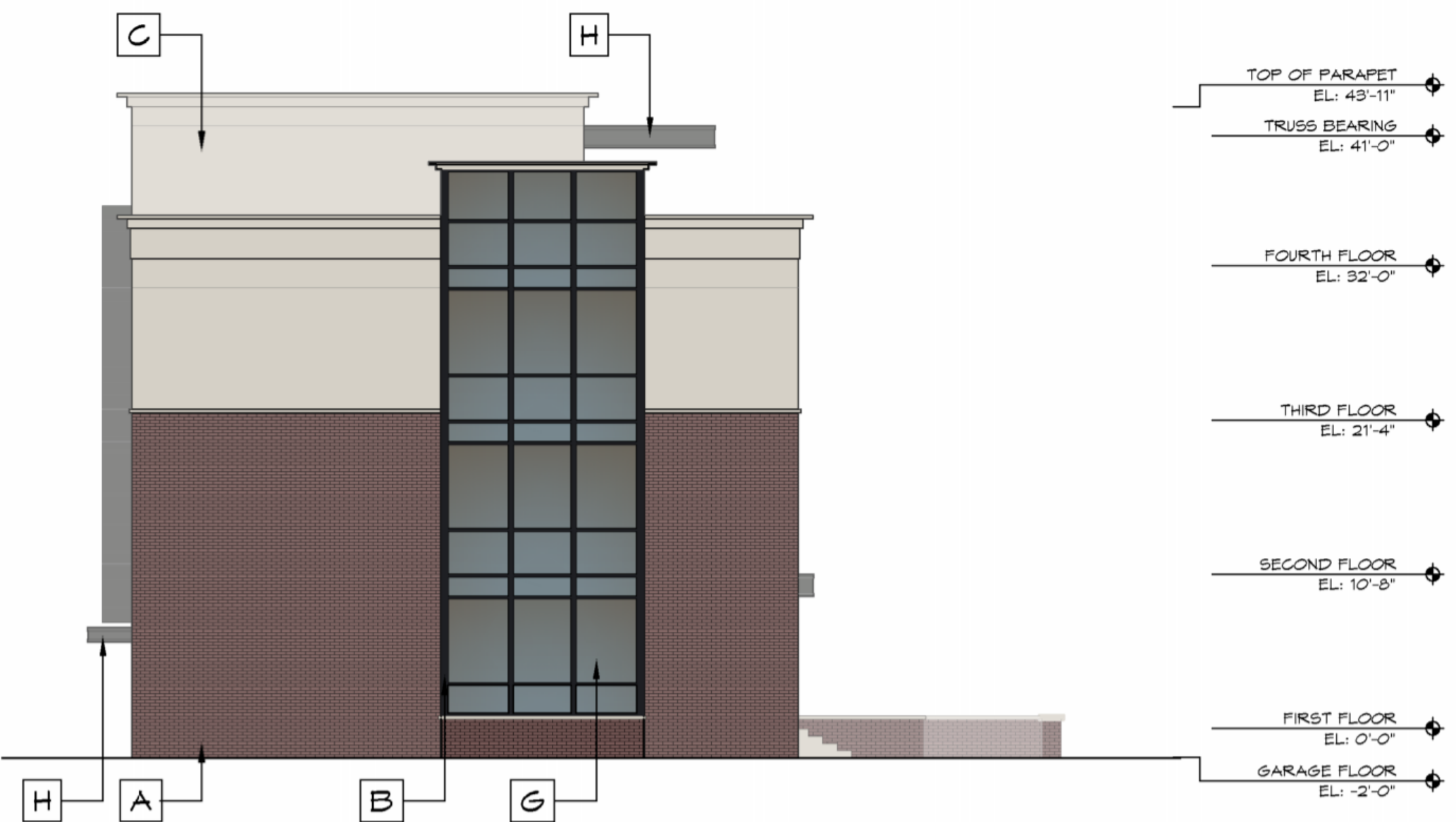
04 | TOWNHOME BLDG TYPE A SIDE ELEVATION SCALE: 1/8" = 1'-0"
