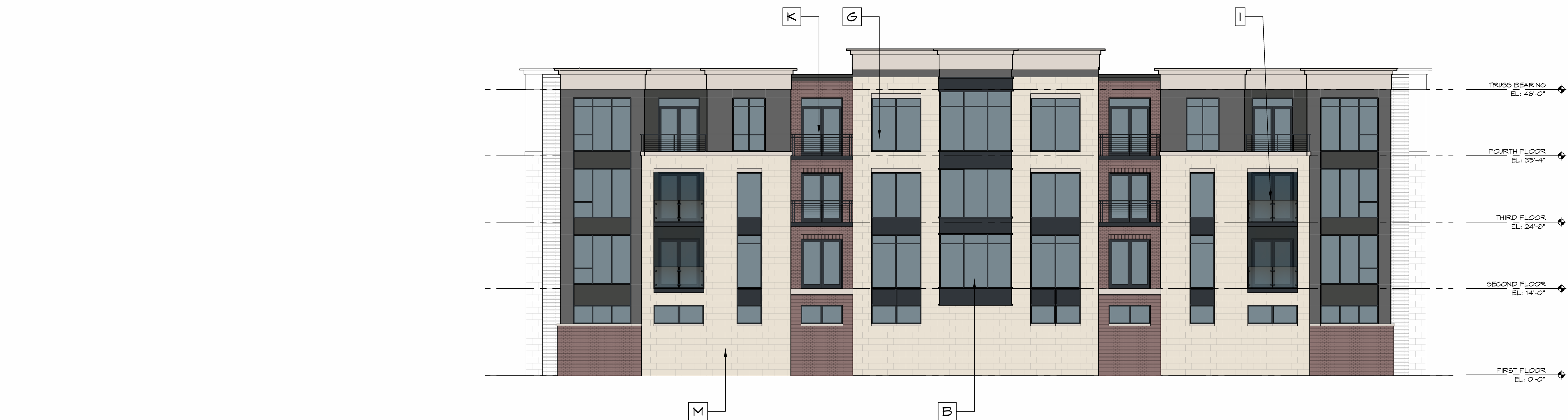
03 APARTMENT BUILDING WEST ELEVATION SCALE: 1/8" = 1'-0"
