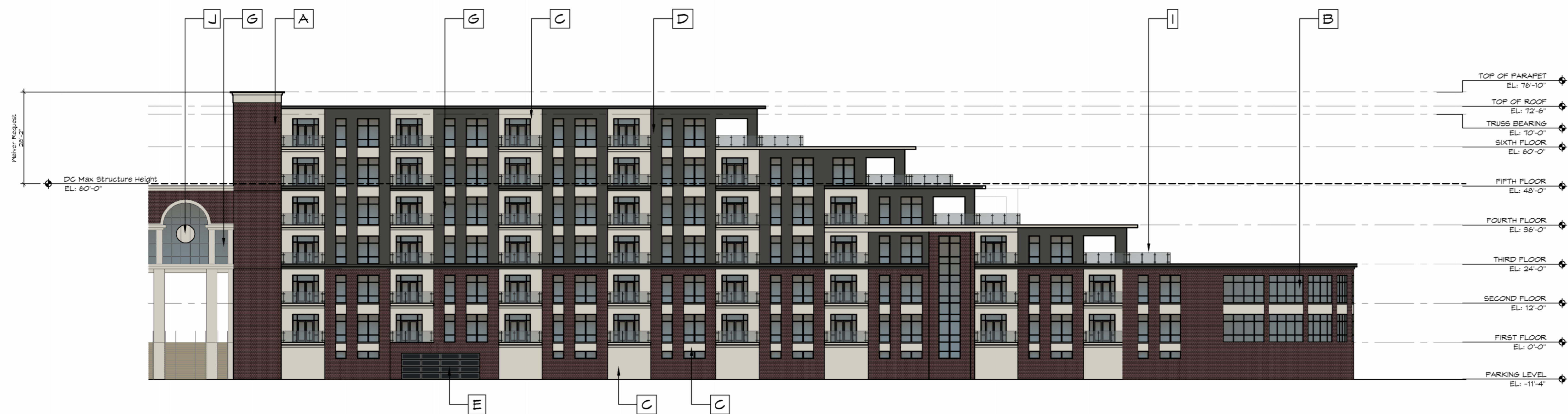
01 CONDO BUILDING C OVERALL COURTYARD SIDE ELEVATION SCALE: 1/16" = 1'-0"
