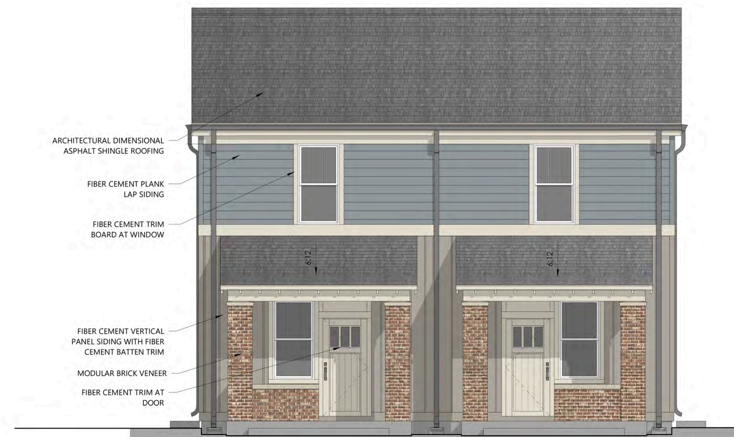
1 FRONT ELEVATION A240-Q 1/4" = 1'-0"
