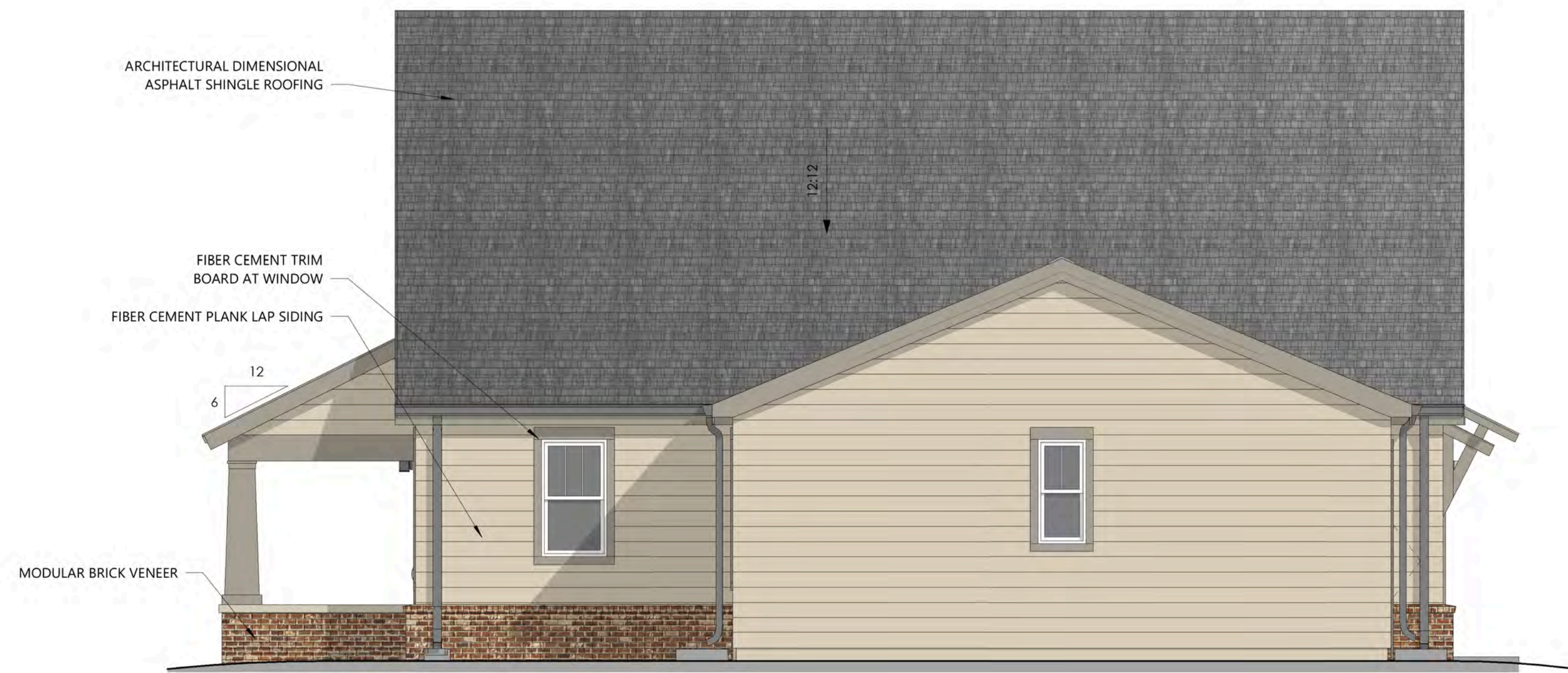
D ELEVATION A217-R 1/4" = 1'-0"
