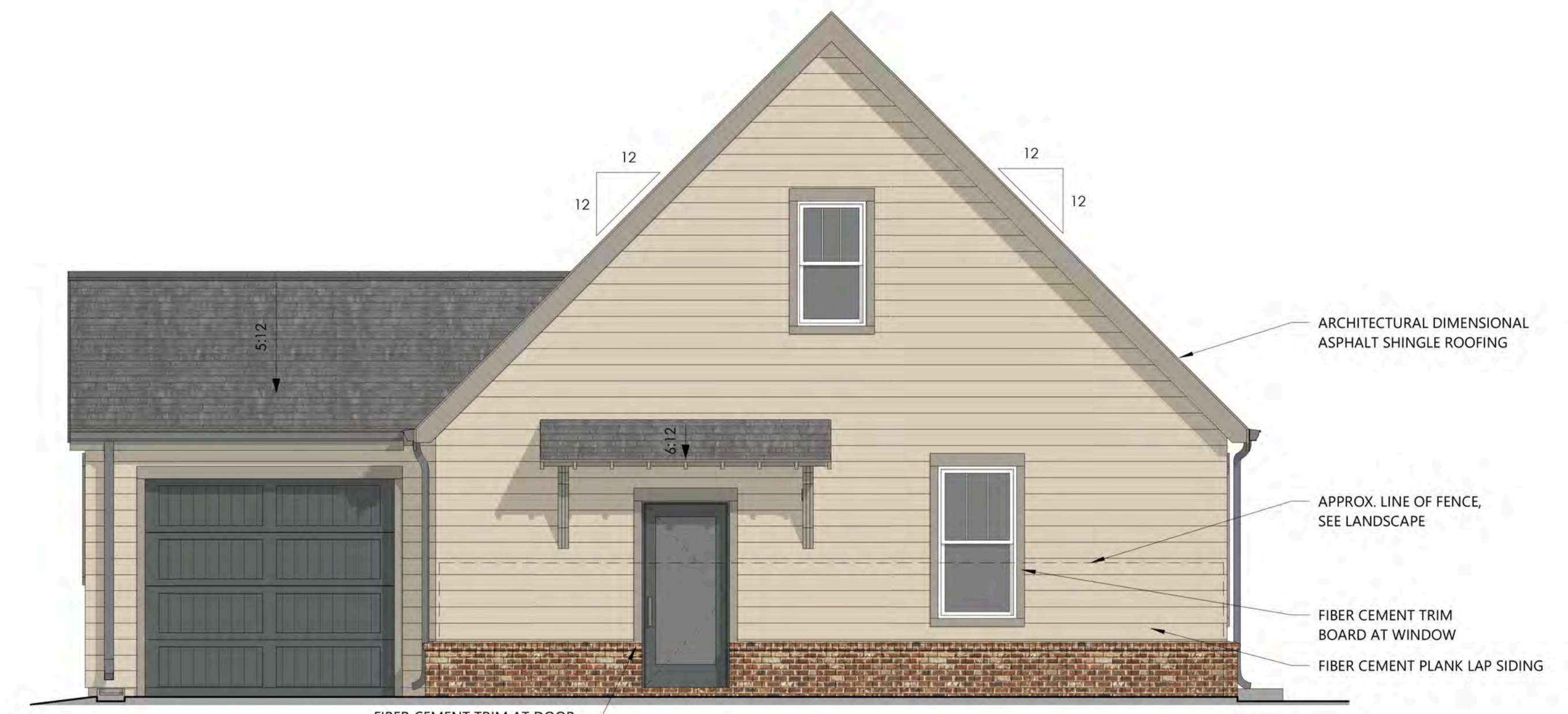
C ELEVATION A217-R 1/4" = 1'-0"
