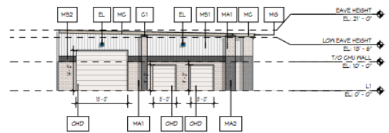
3 SOUTH ELEVATION SCALE: 1/16" = 1'-0"
