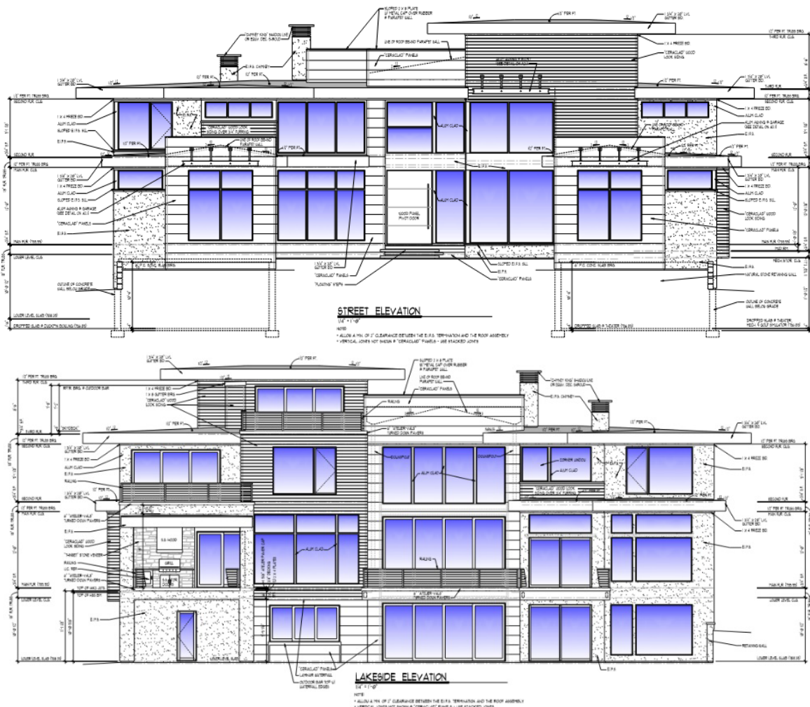
Figure 2. Front and rear elevations of the proposed custom-built home.
