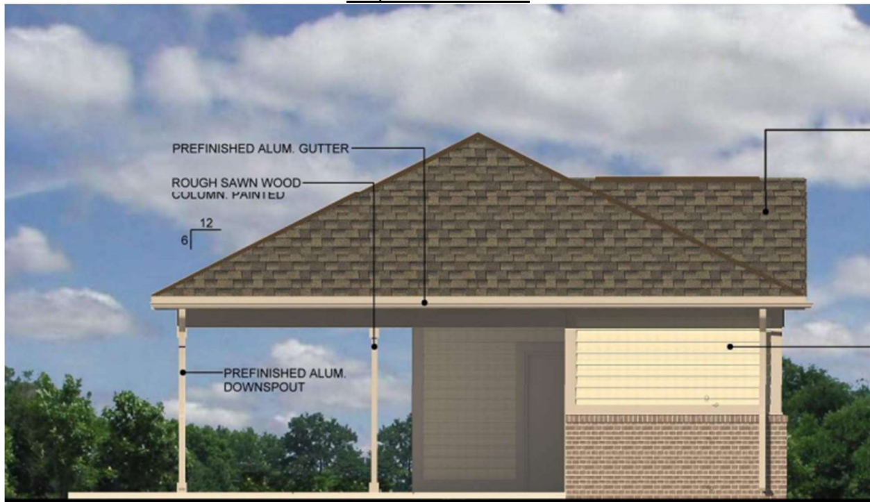
Left side (north) elevation
