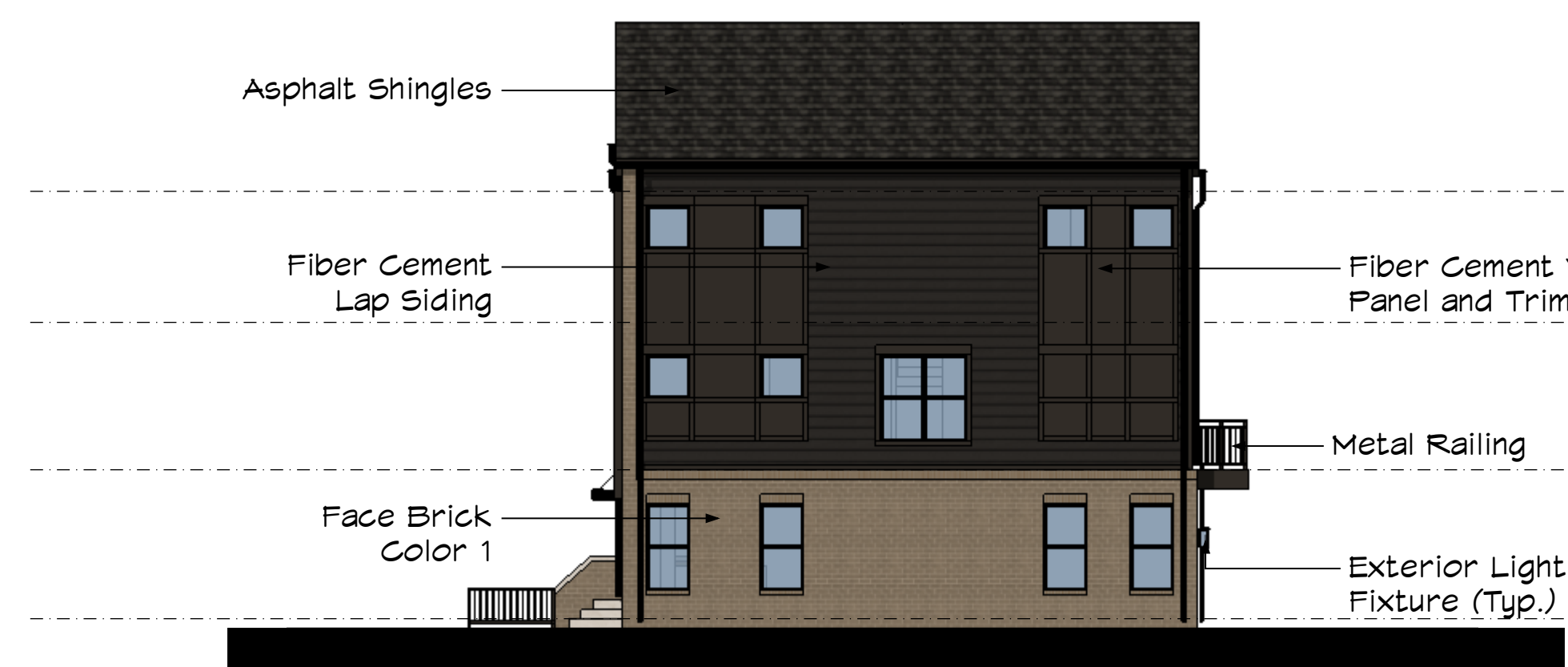
SIDE ELEVATION 1 - 3 UNIT BUILDING TYPE Scale: 3/32" = 1'-0"
