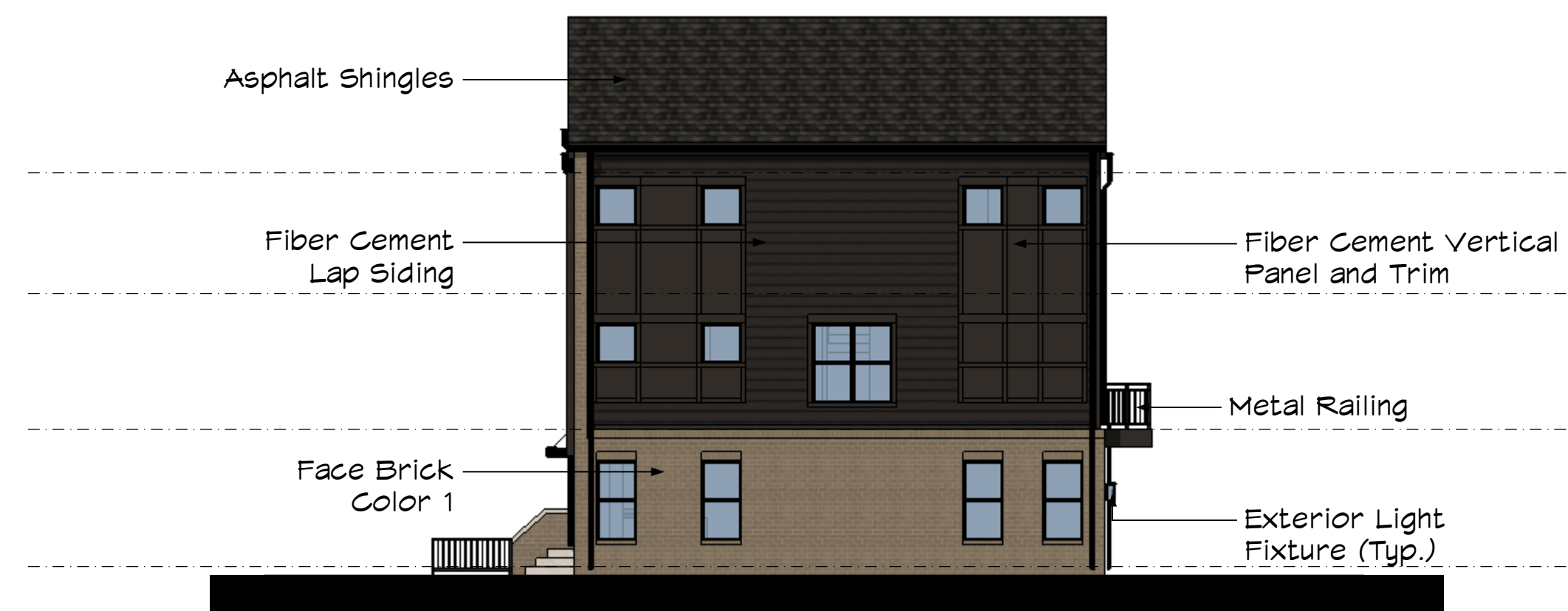
SIDE ELEVATION 1 - 3 UNIT BUILDING TYPE Scale: 3/32" = 1'-0"
