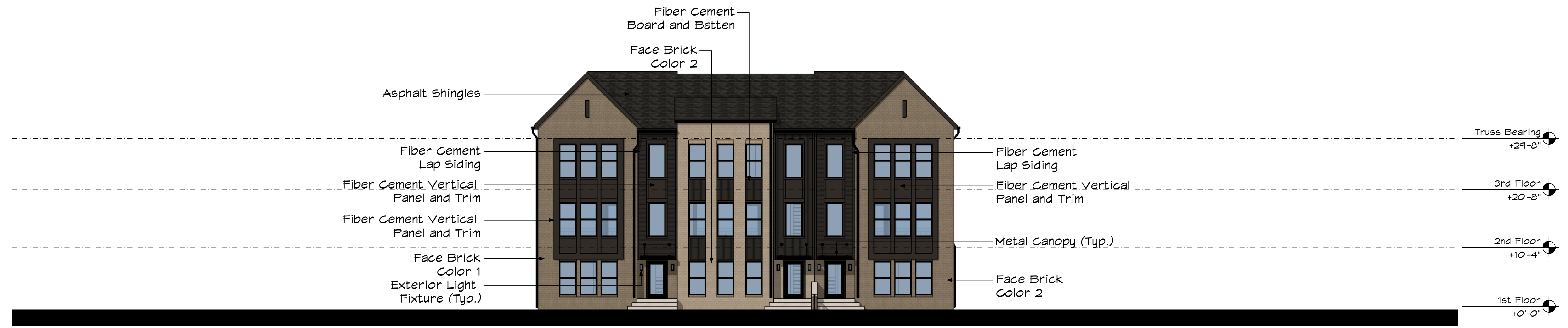
FRONT ELEVATION - 3 UNIT BUILDING TYPE Scale: 3/32" = 1'-0"
