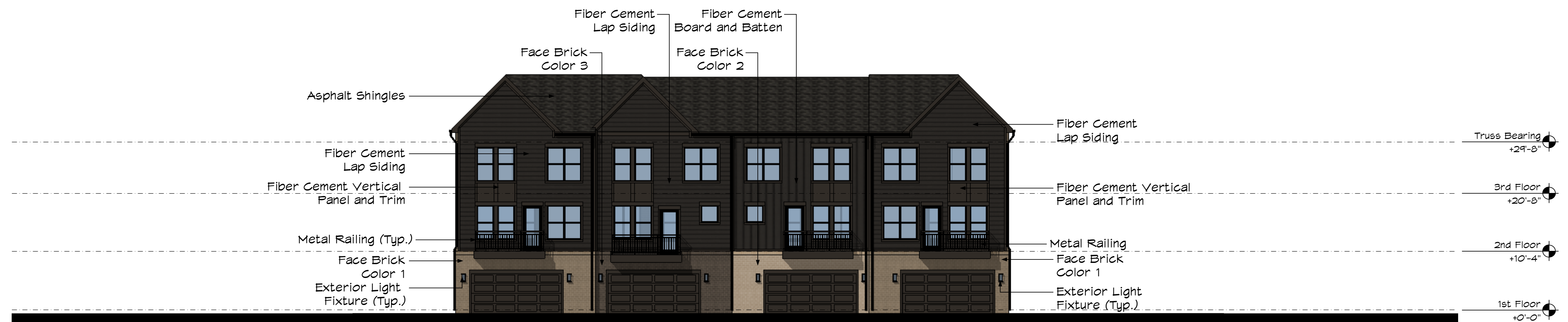
BACK ELEVATION - 4 UNIT BUILDING TYPE Scale: 3/32" = 1'-0"
