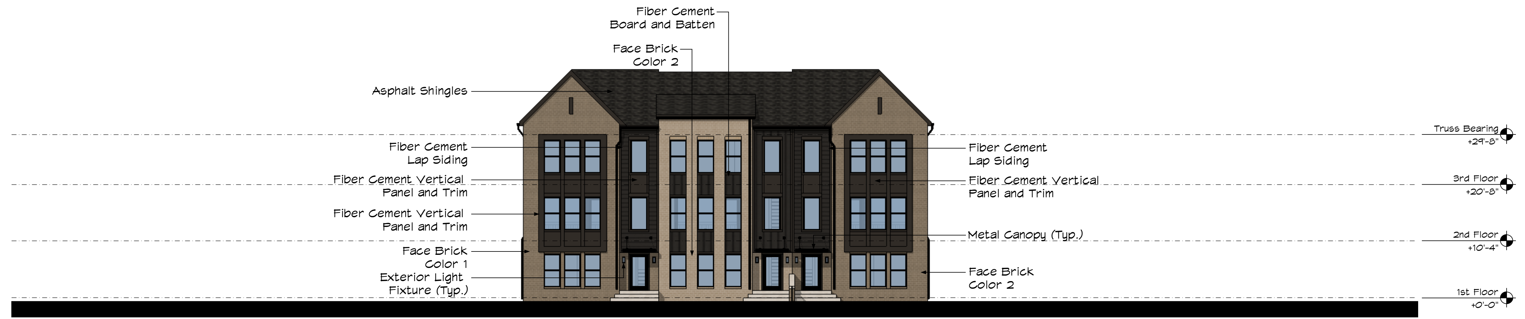
FRONT ELEVATION - 3 UNIT BUILDING TYPE Scale: 3/32" = 1'-0"
