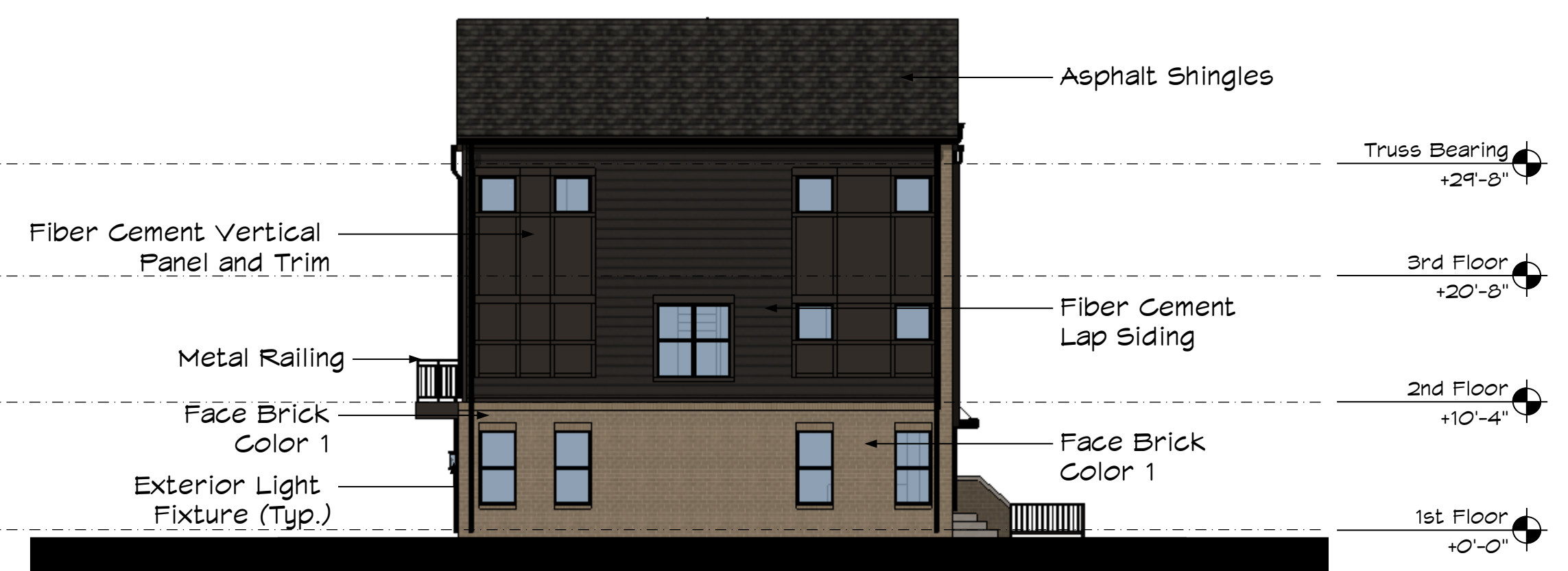
SIDE ELEVATION 2 - 3 UNIT BUILDING TYPE Scale: 3/32" = 1'-0"
