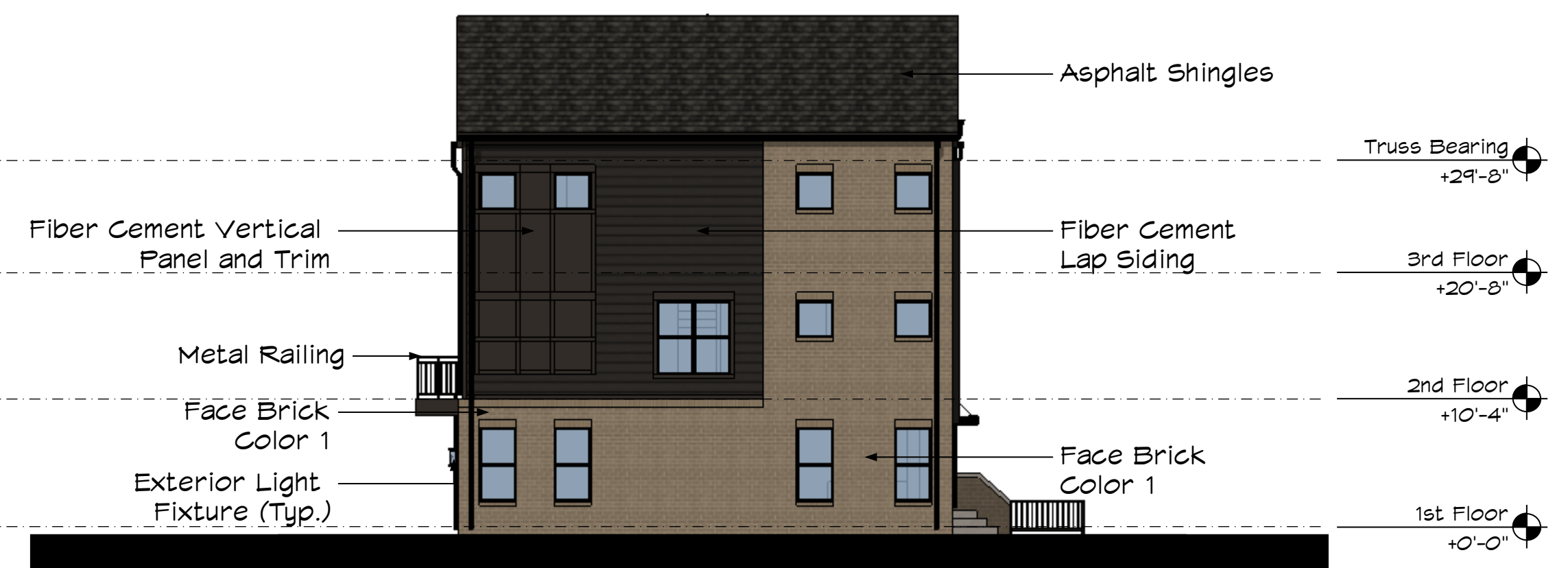
SIDE ELEVATION 2 - 3 UNIT BUILDING TYPE Scale: 3/32" = 1'-0"
