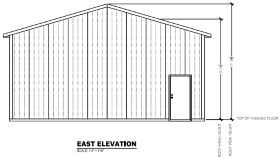
Figure 3. West and East elevations of proposed pole barn.
