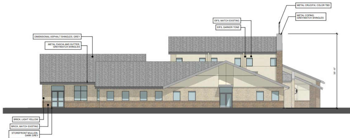
Left side (west) elevation of the addition
