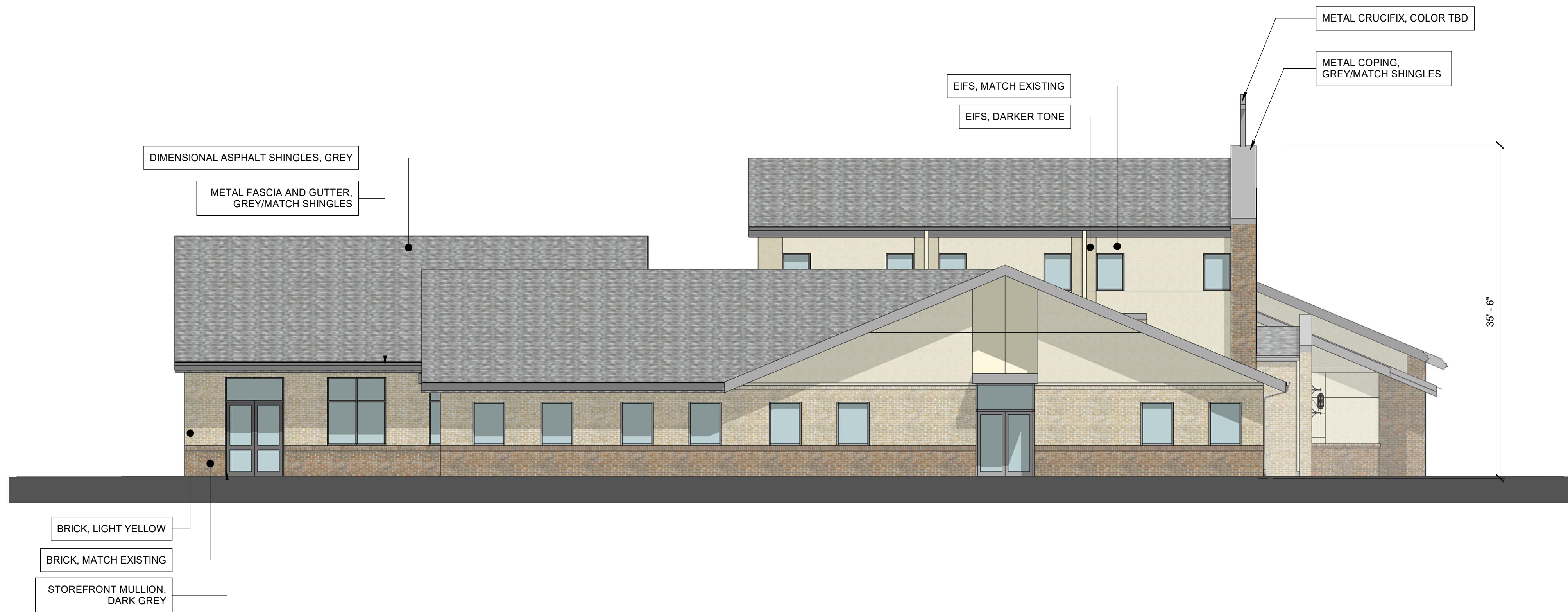
2 Detail West Elevation TAC.2 1/8" = 1'-0"
